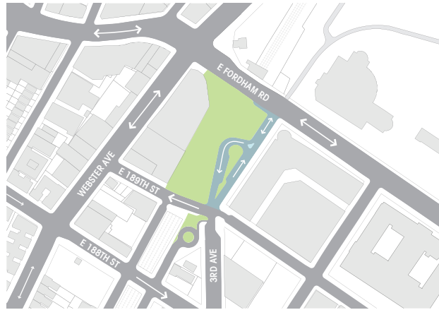
Converting 3rd Ave at the Plaza to bus-only reduces modal conflicts and simplifies the road network, helping reduce traffic congestion. The addition of an extended left-turn lane on Webster improves North-South flows and helps reduce congestion at the Webster/Fordham intersection.
