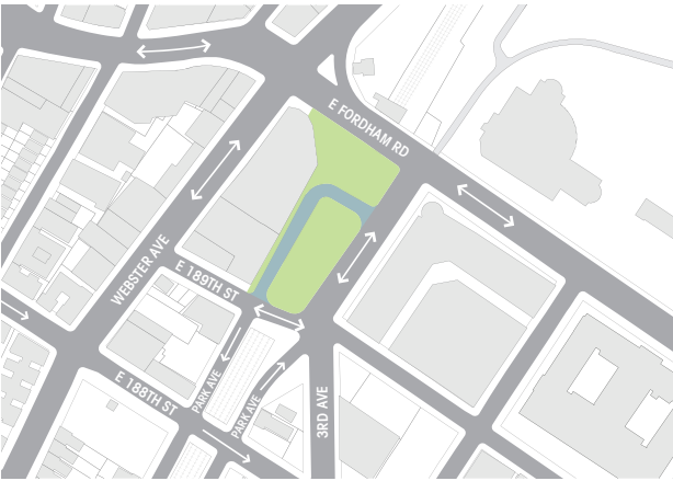
The existing transit exchange bisects the public space of the Plaza, which results in modal conflicts.
